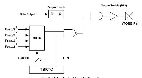
Fig. 7. TONE Output Pin Configuration
